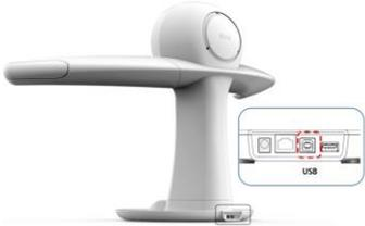
A white RAYFace scanner is shown next to a PC. A red box highlights the USB port on the scanner and the USB port on the PC. A label 'USB' is placed below the PC port.                                                             | RAYFace 와 PC 를 USB 로 연결합니다. |
